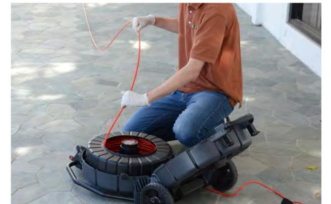
Figure 26 – Rotating the drum to properly wind the push cable
