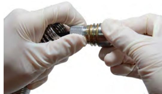
Figure 23 – Removing the camera head
