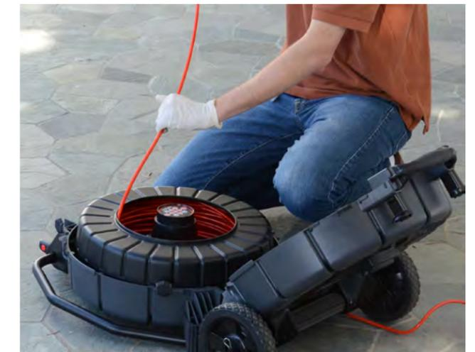
Figure 27 – Guiding the push cable into the drum
