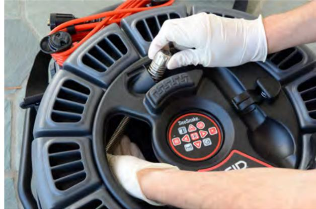
Figure 28 – Routing the camera head
