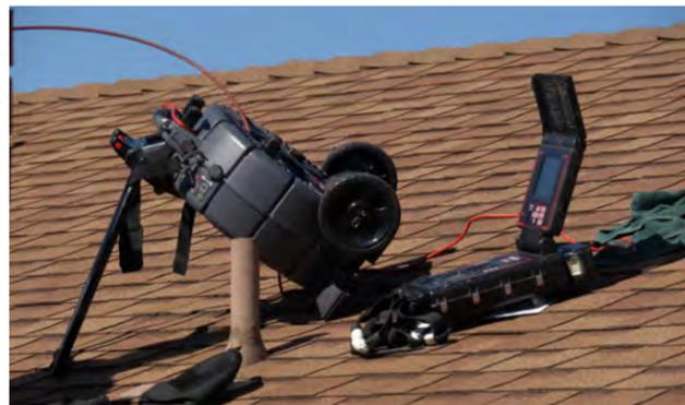
Figure 16 – rM200 and its kickstand during a rooftop inspection
