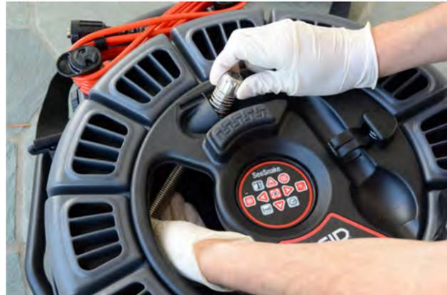
Figure 28 – Routing the camera head
