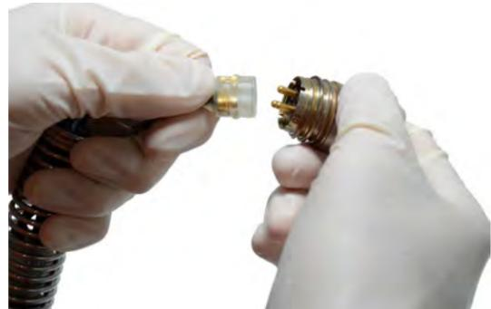
Figure 24 – Removing the connector
